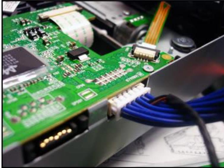
4.) Connect a Molex Connector (=Powercable in the PC) from the PC to the CK3
